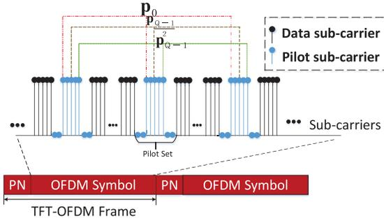
Fig. 1. TFT-OFDM signal structure with the proposed pilot pattern.
